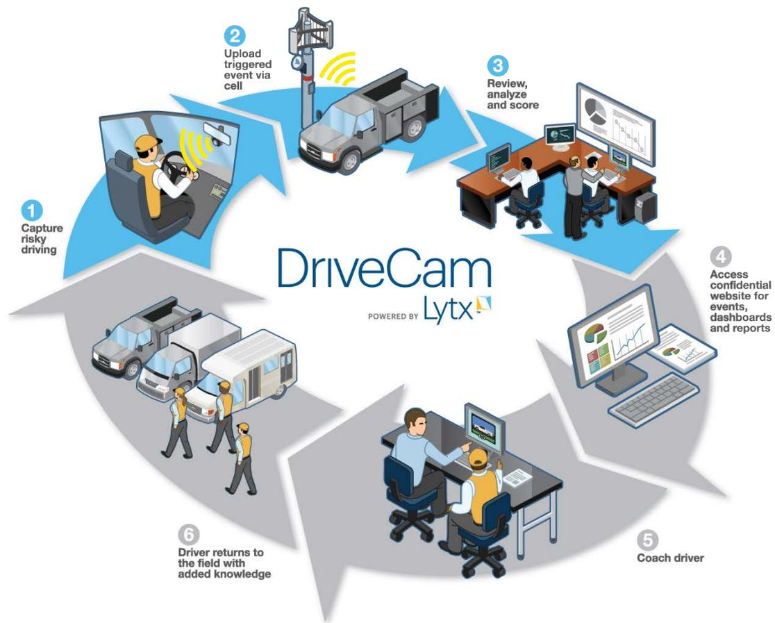
**Figure 1. Illustration. Schematic of the DriveCam® program**
